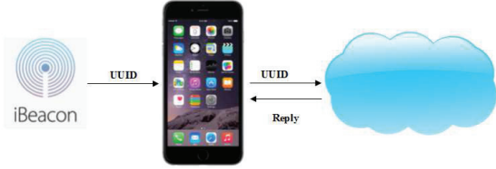
Fig. 1. Working principal of the iBeacon
